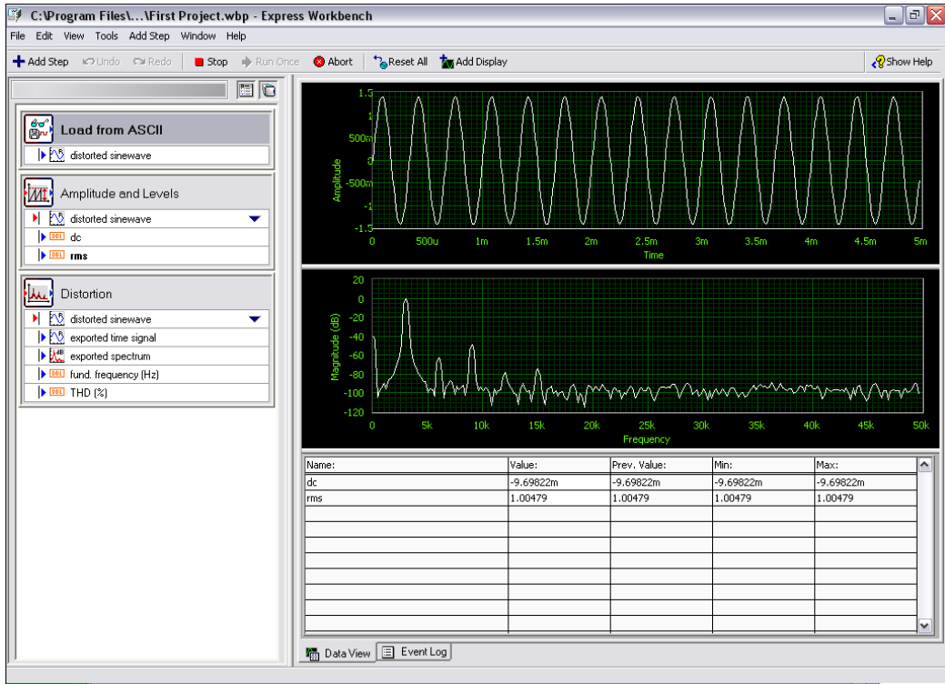
Figure 3-2. Outputs of First Project.wbp
